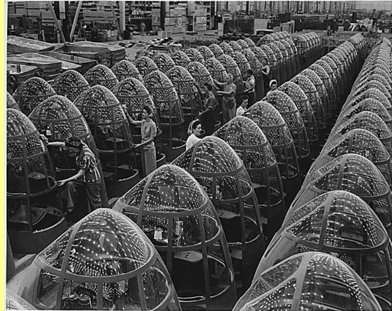
Factory workers polish Plexiglas nose cones for A-20 attack bombers
